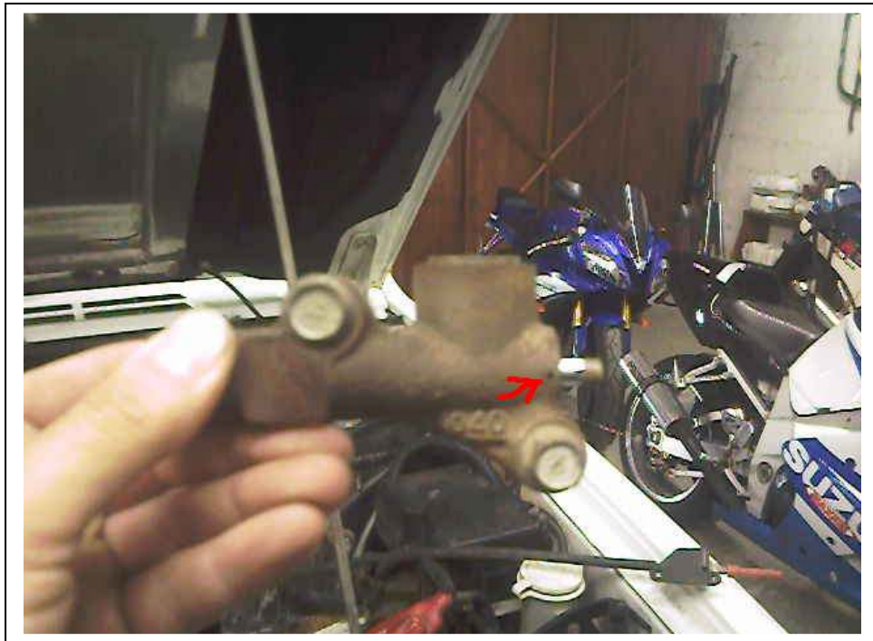
This is the auto tensioner removed note the small hole.
