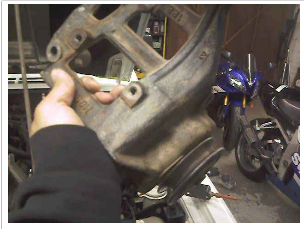
This is the aircon bracket removed.
