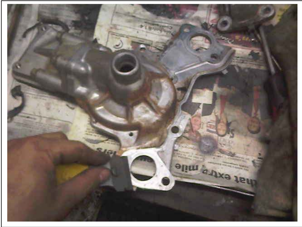
Cleaning the surfaces of the water pump housing
